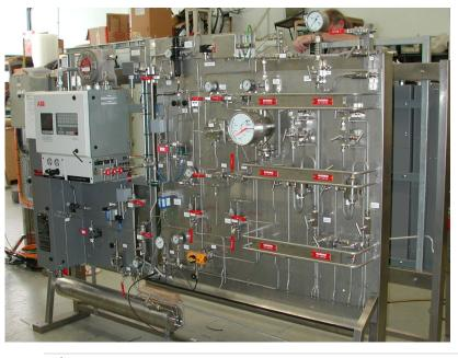
Process analyzers are online tools for industrial process analytics, used to determine the chemical composition or physical properties of substances involved in industrial processes. They enable process optimization, asset protection, and compliance with environmental regulations.
